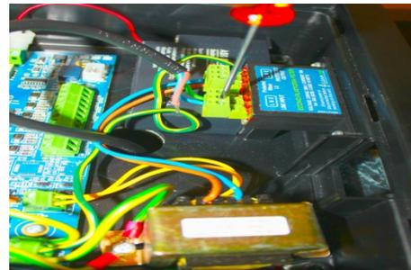
**Figure 20: Connecting 220V**
