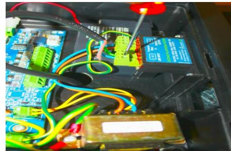
**Figure 11: Connecting 220V**
